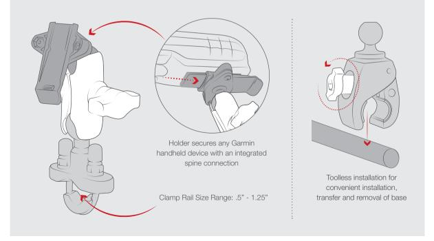
RAM-B-202-GA76U RAM<sup>®</sup> Spine Clip Holder with Ball for Garmin Handheld Devices
