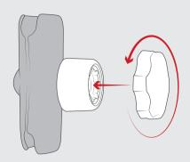
The RAP-S-KNOB5U offers the ideal amount of leverage to properly tighten your mount to prevent slippage in heavy chop or in extreme vibration environments.
