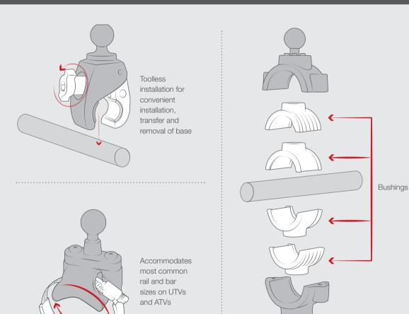
Internal bushings conform to your handlebar while protecting the surface
