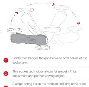
the end sockets, allowing you to pivot the ball and socket connection. Stainless steel and nylon washers ensure smooth and 4 secure friction when tightening your mount.
