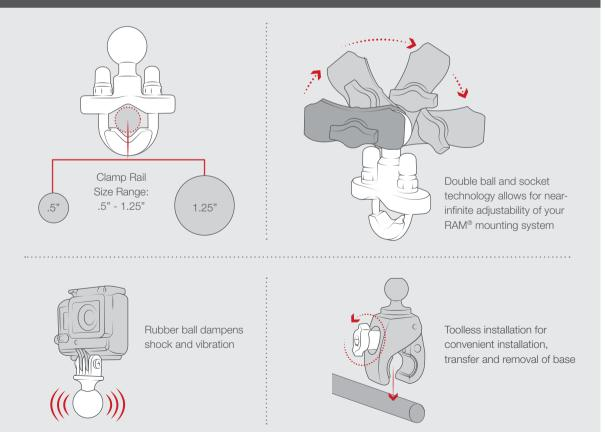
RAM-B-149Z-SP06U RAM<sup>®</sup> EZ-Roll'r<sup>™</sup> Handlebar U-Bolt Mount for SPOT Gen4
